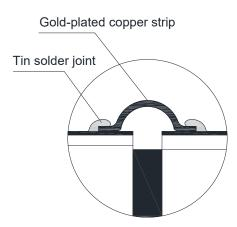
b, the use of gold belt/wire bonding interconnect, the width of the gold belt is less than the width of the microstrip circuit, no multiple bonding is allowed, the bonding quality should meet the requirements of GJB548B method 2017.1 Article 3.1.5, the bonding strength should meet the requirements of GJB548B method 2011.1 and 2023.2.
